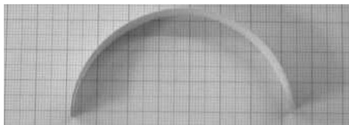
*Flexibility gives the coating resilience against small impacts or deformation of the substrate. Avoids cracking in-service*
