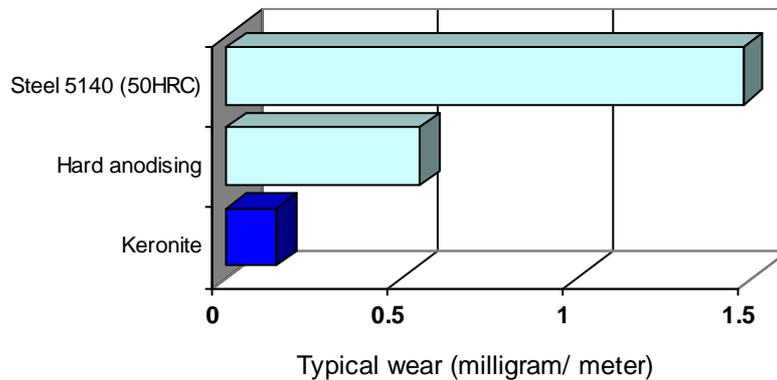
*The wear resistance of Keronite was evaluated by the pin-on-disk method and compared with the wear resistance of hard anodic coating (Mil-C-8625 type 3) and of 5140 steel 50 HRC*
