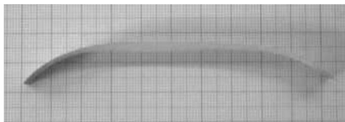
*100µm detached Keronite film showing ability to be bent or flattened elastically. In more severe deformation, both plastic and elastic deformation occurs before failure*
