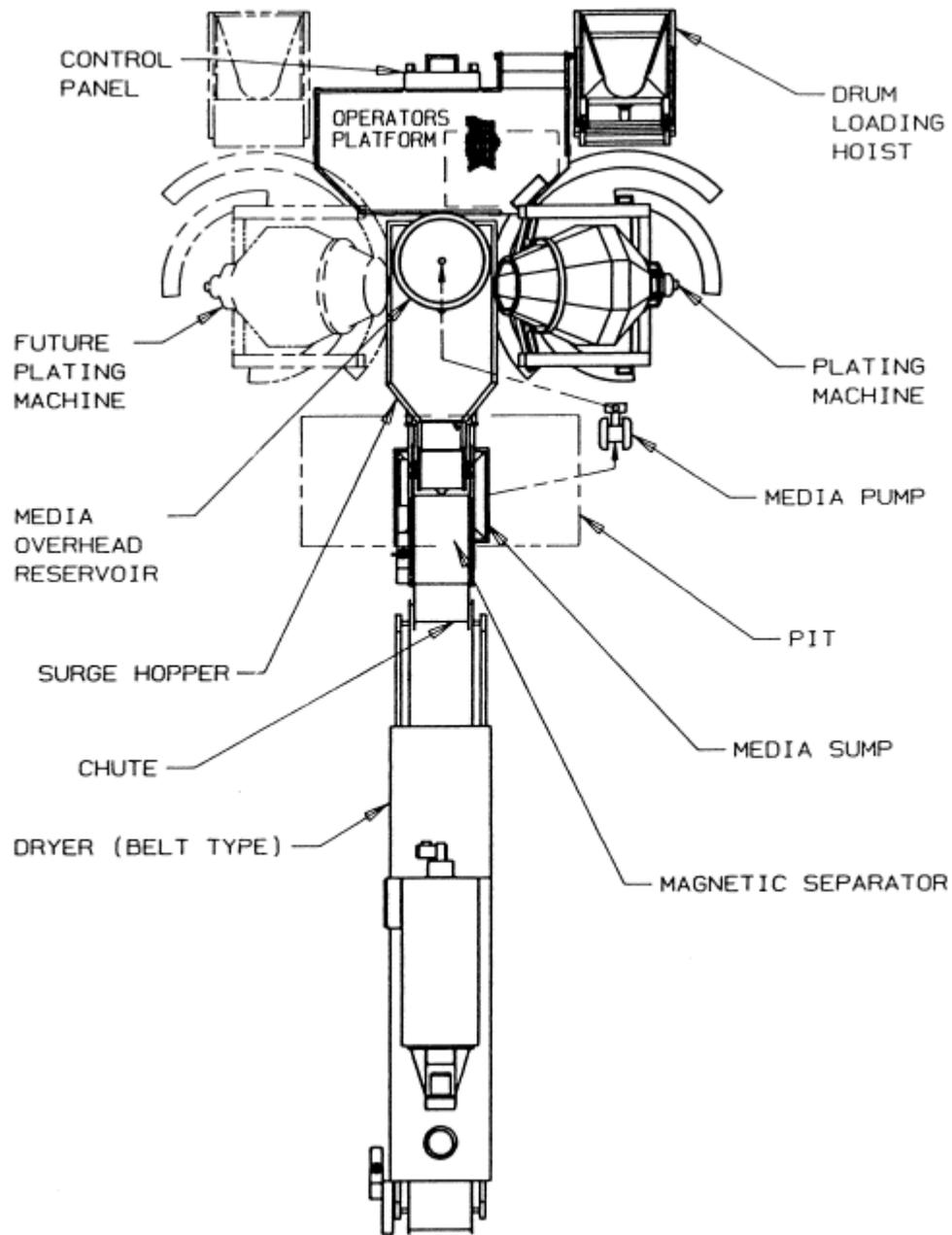
Fig. 3 - The Alloy MP-ACQ fastener coating system equipment.
