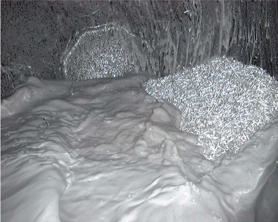
Fig. 1 – Co-deposited matrix of metals and linking agents applied by physically mixing them in a aqueous slurry.
